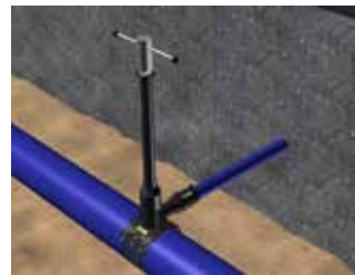
Figure C.41: Tapping of the pipe
