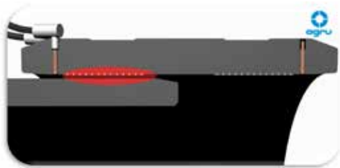
Figure C.18: Principle of the bifilar welding
