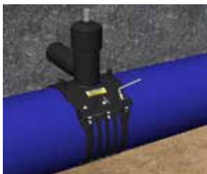
Figure C.39: Mounting the pressure tapping valve
