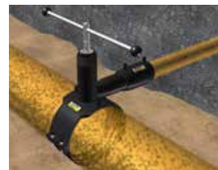
Figure C.36: Tapping of the pipe
